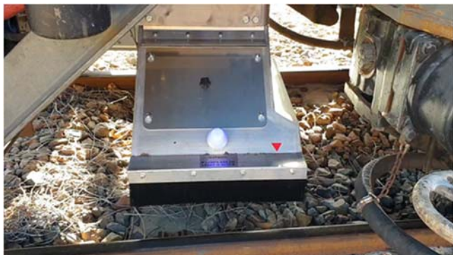
Figure 9 ATIS Track Geometry unit mounted to diesel locomotive
