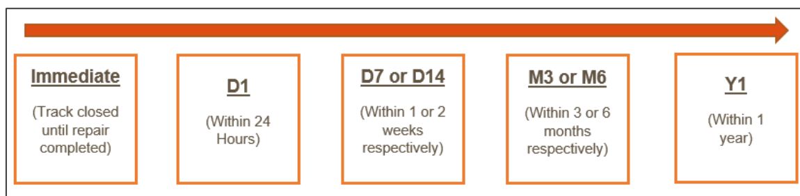
Figure 90 Timeframes associated with corrective maintenance activities
