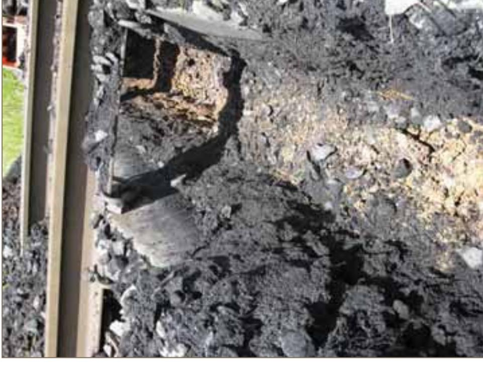
Sampling of Ballast by Destructive Means
