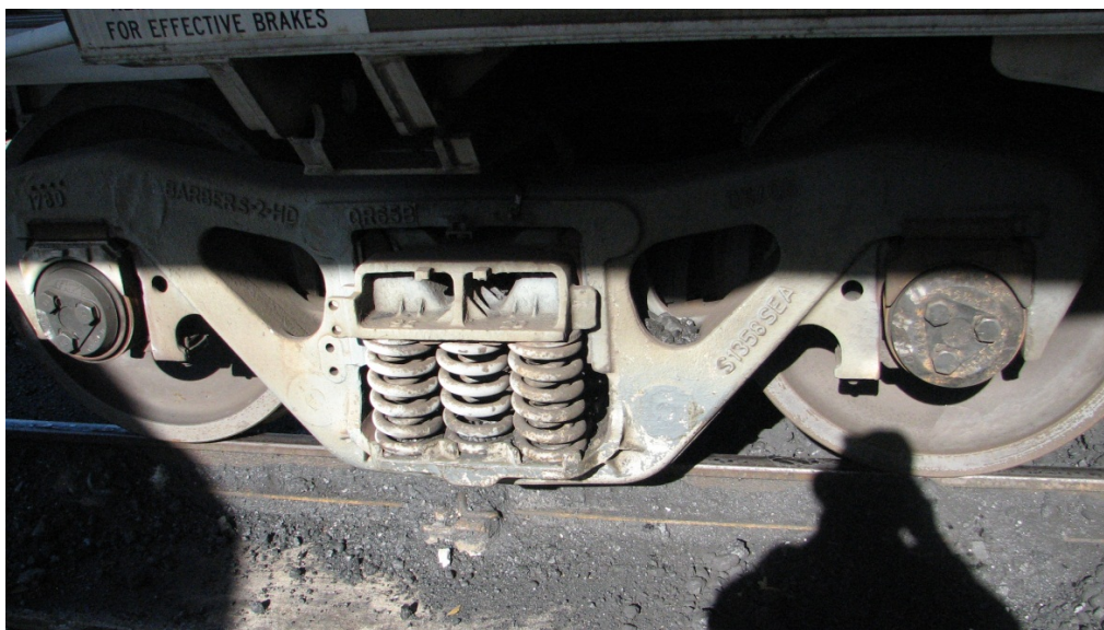
Figure 4: Example of parasitic coal on a wheel bogie
