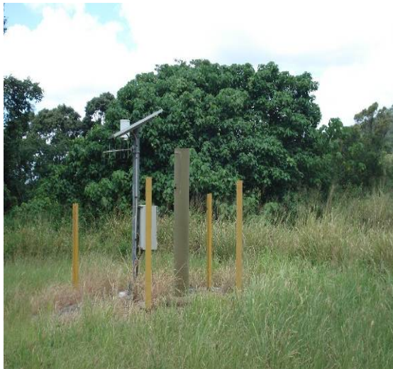
Figure 4: Rainfall density measurement
