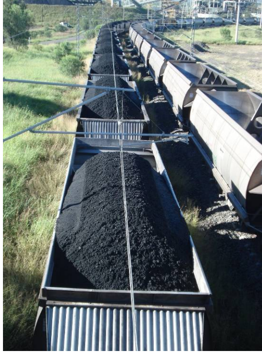
Figure 4 Wagon overloaded spillage occurring
