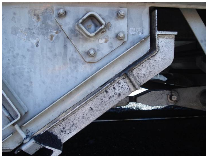
Figure 9 Gap and residual fines left on the bottom of wagon on completion of unloading process
