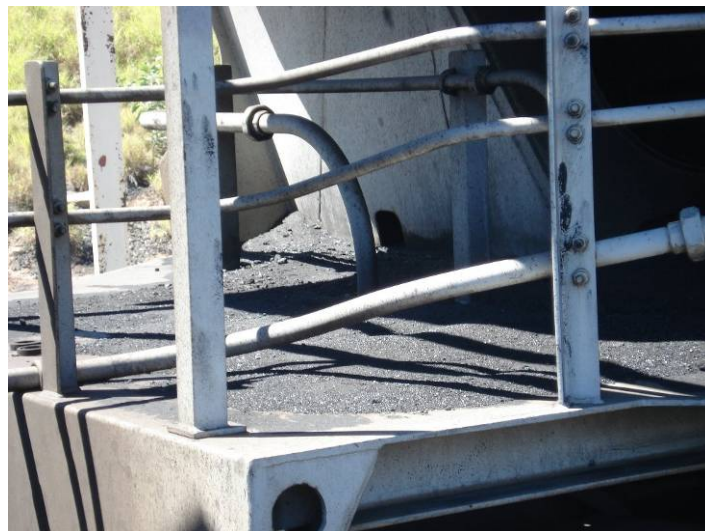
Figure 6 Spillage on wagon platforms can easily be blown or shaken off on route – this was commonly sighted
