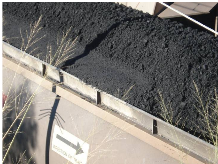
Figure 3 Some wagons were altered with an addition of a metal strip to allow additional loading capacity, as can be noted spillage is already occurring from this wagon
