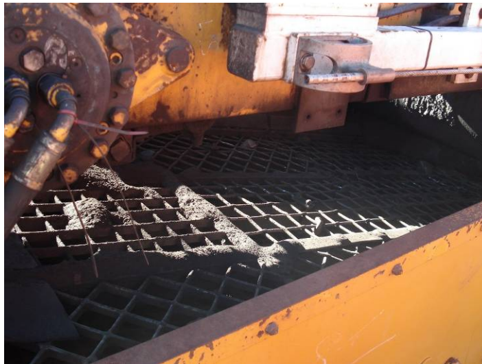
Figure 13 Screen for separating the fine parts and damaged ballast from reusable ballast
