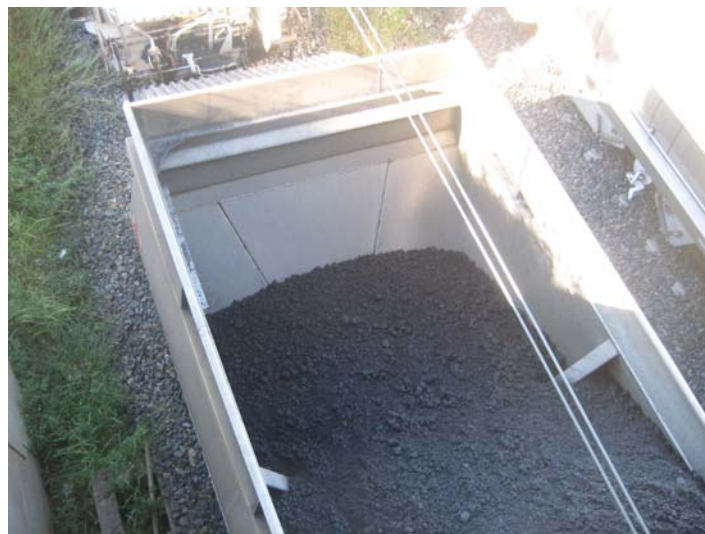
Figure 1 Wagons were found to be often heavily loaded at the front of the car whilst empty at the back
