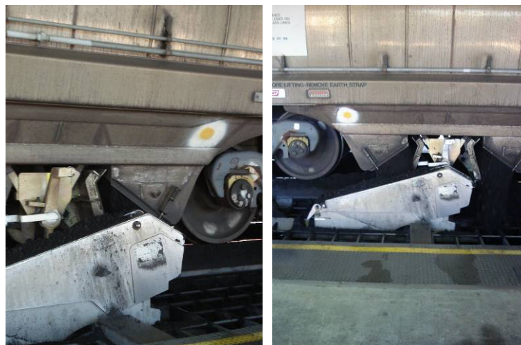
Figure 7 Unloading with mechanical barrier
