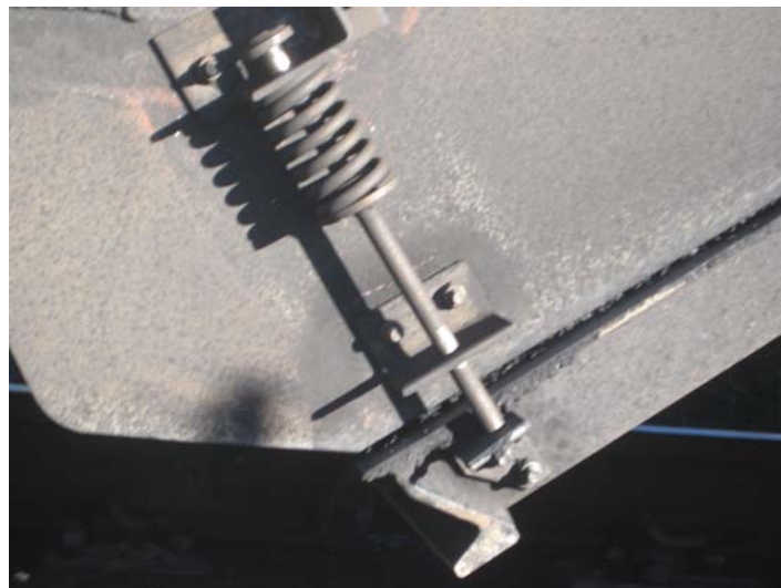
Figure 2 Wagon C, substantial fines were seen falling from these gaps which appeared to be in the range of 5-20mm
