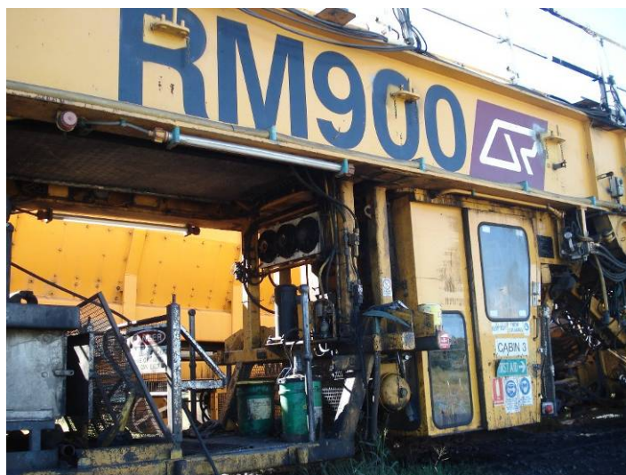
Figure 11 The machine has a ballast cleaning capacity of 900m 3 per shift
