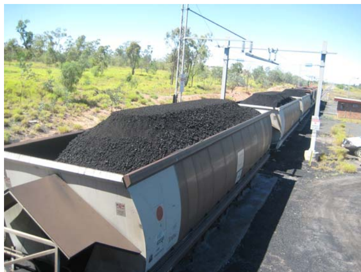
Figure 8 Coal left on edge of wagon from loading process
