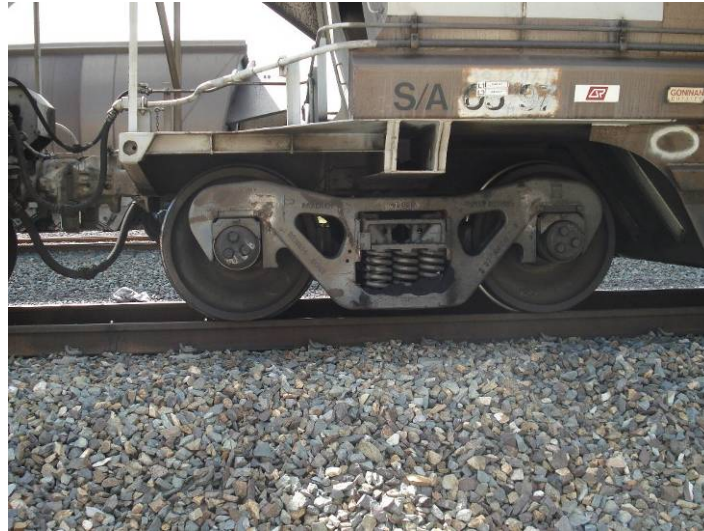
Figure 6 Coal dust on wheel set springs after loading process
