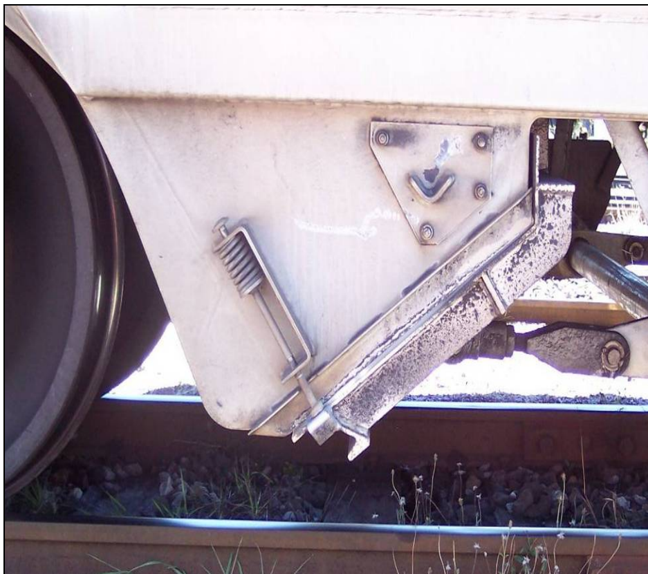
Figure 6 Gaps on wagon bottom doors allow spillage in transit
