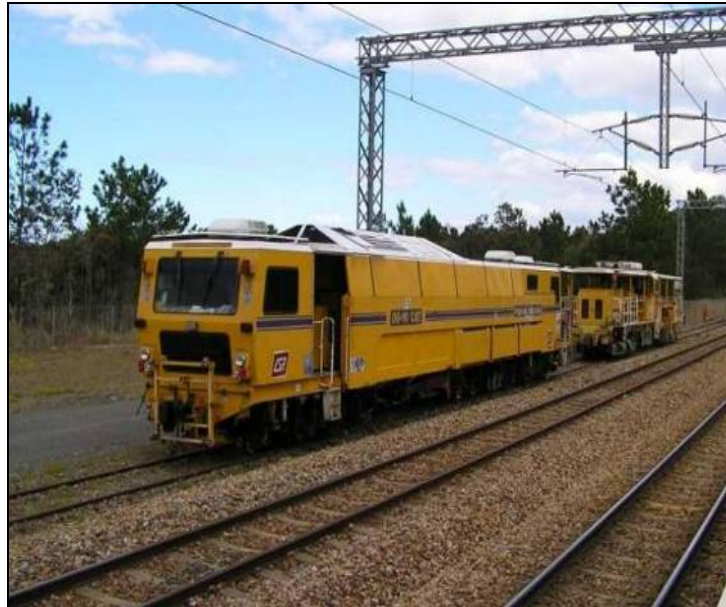
Figure 39 QR Ballast Tamper and Ballast Regulator
