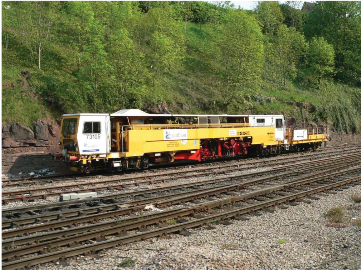
Figure 17: Ballast tamping machine
