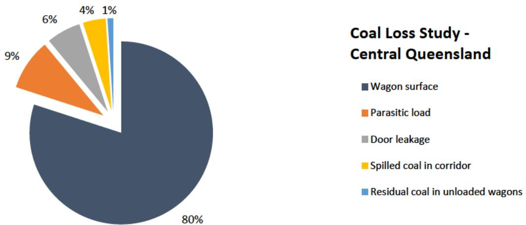
Figure 3. Sources of Coal loss
